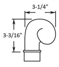
This decorative brass finial is made of brass and has a polished finish. It is to fit into tube with a 2" outside diameter and a 0.05" wall thickness.
