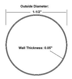
00-A110 architectural round tube is a brass tube with a 1-1/2" outside diameter, a 0.05" wall thickness, and is available in stock lengths up to 16 feet. It is made with C2680 alloy brass and conforms with ASTM B36.
