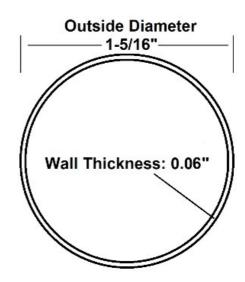
The brass finish A106 premium closet rod is made of quality steel with a durable brass plated finish. Outside diameter is 1-5/16" and wall thickness is 0.06".
