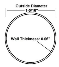
The white finish A106 closet rod is made of quality steel with a durable plated finish. Outside diameter is 1-5/16" and wall thickness is 0.06".
