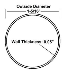
The satin (brushed) stainless finish A106 premium closet rod is made of quality steel with a durable stainless steel outer layer. Outside diameter is 1-5/16" and wall thickness is 0.05".
