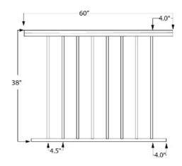
This 5ft long Level Picket Rail Panel is designed for 42" high railing and it has 3/4" square pickets that are spaced 3-3/4" apart to pacify the 4" sphere rule. This panel has a white painted finish.
