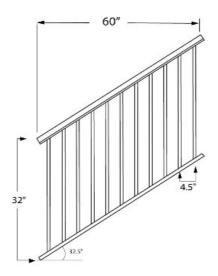
This 5ft long Stair Picket Rail Panel is designed for 36" high railing and it has 3/4" square pickets that are spaced 3-3/4" apart to pacify the 4" sphere rule. This panel has a dark bronze painted finish.
