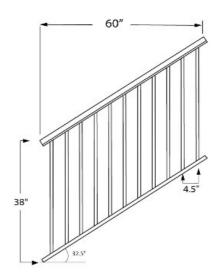
This 5ft long Stair Picket Rail Panel is designed for 42" high railing and it has 3/4" square pickets that are spaced 3-3/4" apart to pacify the 4" sphere rule. This panel has a white painted finish.
